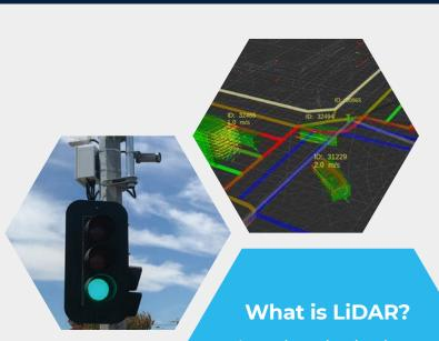
Laser-based radar that captures millions of 'points' of information in 3D space that collectively are converted to object models for a centimetre-accurate view of every moving and stationary object.
